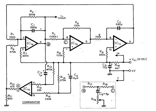
oscillation. Sinewave amplitude is stabilized by virtue of the constant square wave input and is typically  $0.25V_{cc}$  pk-pk, its purity being proportional to filter Q.
