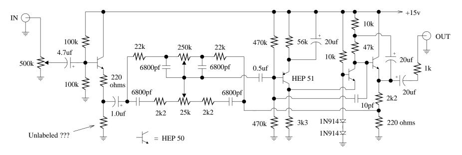
Tone Control circuit with signal isolation and impedance-matching stages.
