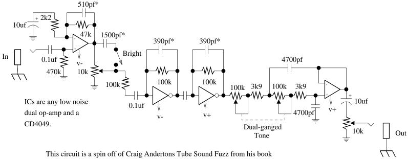
This circuit is a spin off of Craig Andertons Tube Sound Fuzz from his book Electronic Projects for Musicians. This only uses 2 stages of a CD4049 hex inverter/buffer the rest were left out of the schematic to keep it simple. Components with a \* are suggested values, substitutions can be made freely within 30%.
