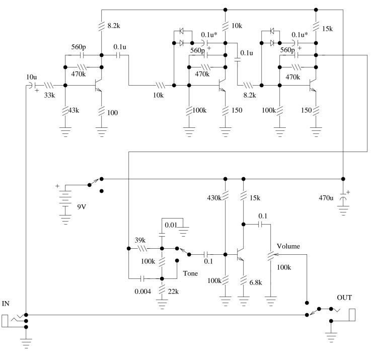
The EH Little Big Muff could probably be improved with modern input jack power switching and a DPDT bypass.
